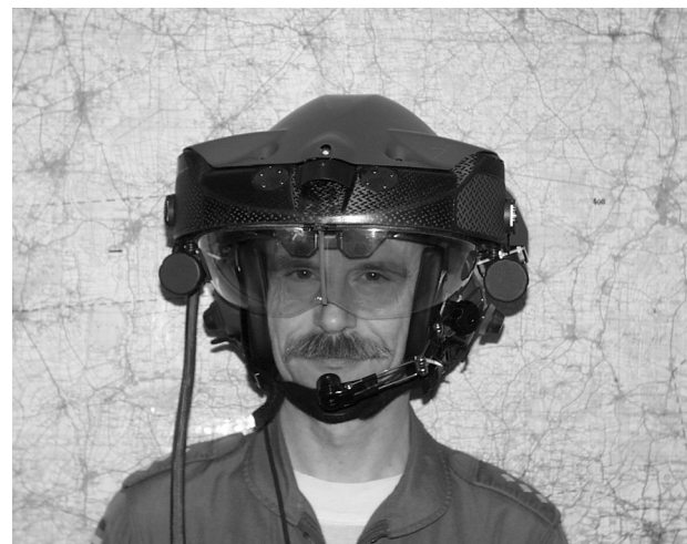
Fig. 8 The TopOwl see-through HMD, designed for helicopter piloting. (View this art in color at www.dekker.com .)
