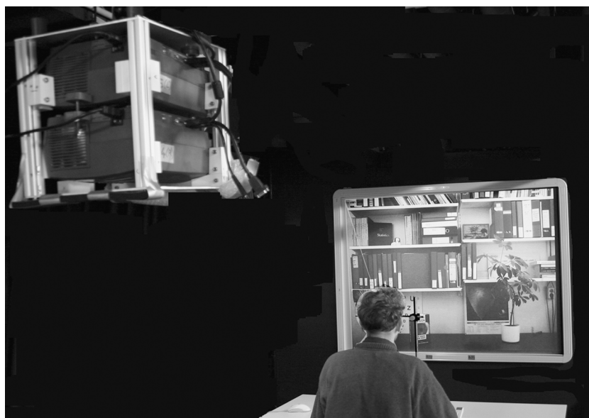
Fig. 9 Two projectors (upper left) equipped with linear polarization filters project the corresponding left- and right-eye images simultaneously on the screen. The subject views the screen ( 170 \times 128 cm) from 185-cm distance through two polarization filters such that the left and right eyes see a separately projected image. With this setup, nearly all binocular errors can be simulated. (View this art in color at www.dekker.com .)
